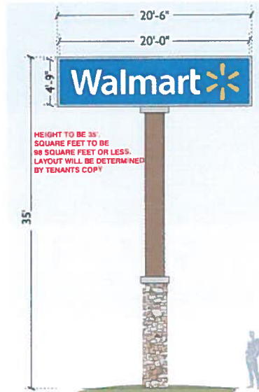
T3 Single Tenant Pylon SCALE: 1/8" = 1'
