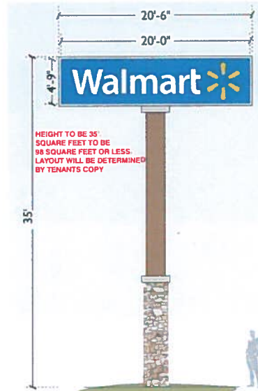
T3 Single Tenant Pylon SCALE: 1/8" = 1'
